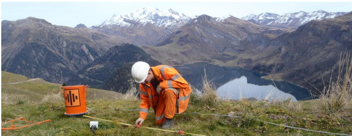
Accurate and reliable knowledge of ground stiffness is key to the economical design of foundations to civil engineering structures. Ground stiffness has traditionally been measured either by crude field testing combined with questionable empirical relationships; laboratory testing of typically unrepresentative soil samples; or for the largest projects using expensive full scale load tests or complex and time consuming insitu measurement techniques.
